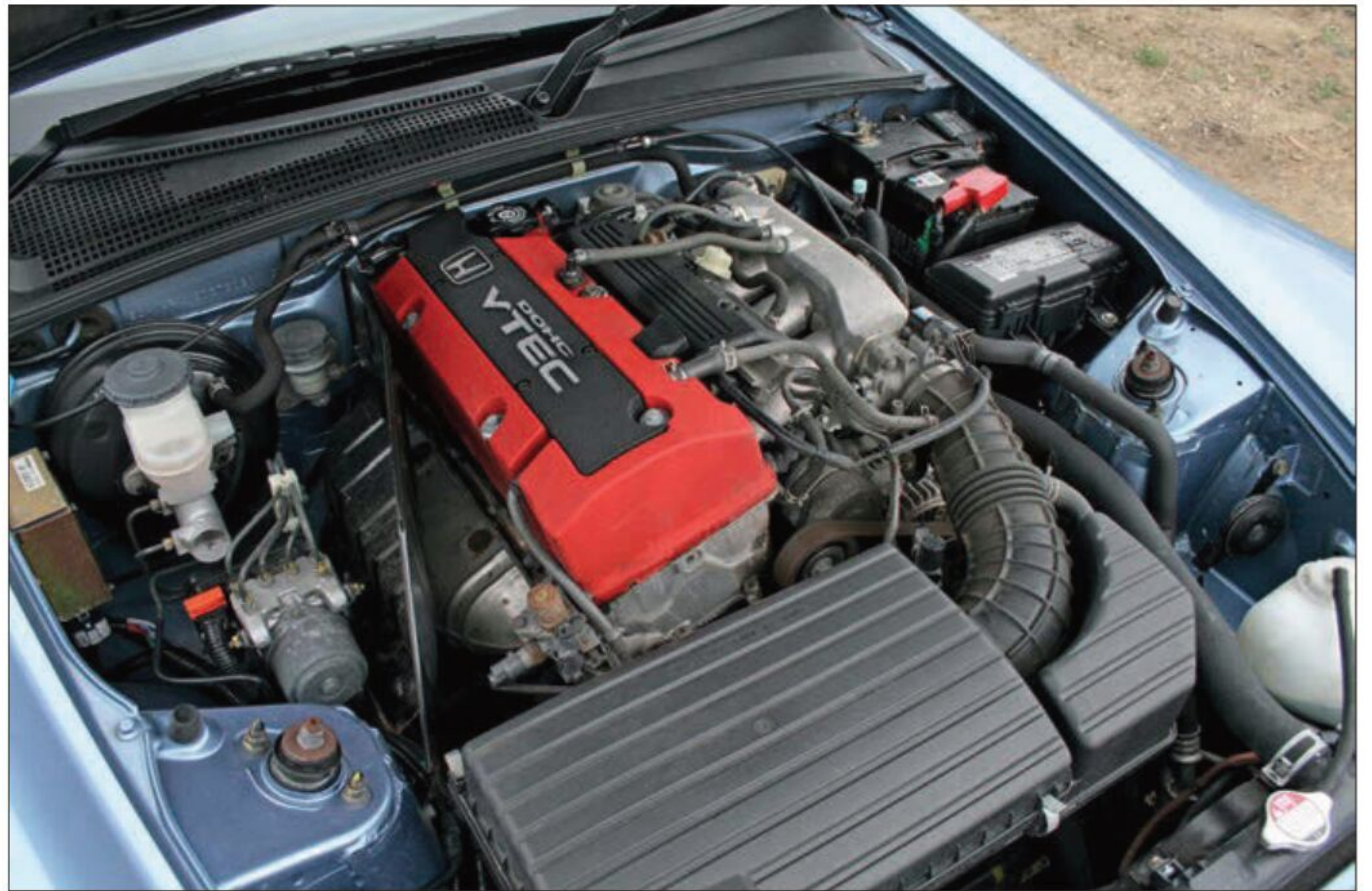
S2000 offers 237bhp from just two litres courtesy of VTEC acting on both cams.
